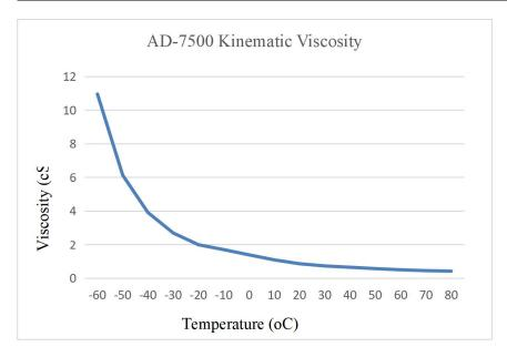
To determine the viscosity at a given temperature T in Kelvin, calculate  $Z = 10^{(10^{(10^{(11.843-5.0874*Log(T[K]))})}$ . Then, Viscosity [cSt] = (Z-0.7) - exp (-0.7487 - 3.295(Z-0.7) + 0.6119(Z-0.7)<sup>2</sup> - 0.3193(Z-0.7)<sup>3</sup>)
